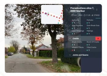
**Borut Hojnik:** "Due to the algorithm, the existing damages are recognized and classified directly while driving around the city with the vialytics system. If we want to analyze the data afterwards, all we need to do is look at the web system. There we can easily monitor all road sections, paired with the individual damages and we don't have to be on site every time.
