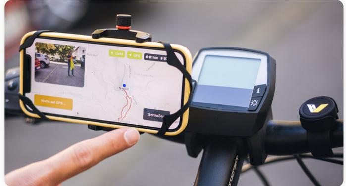
*The vialytics system enables digital road inspection on foot as well as in the car or on a bicycle using a smartphone and steering wheel button.*
