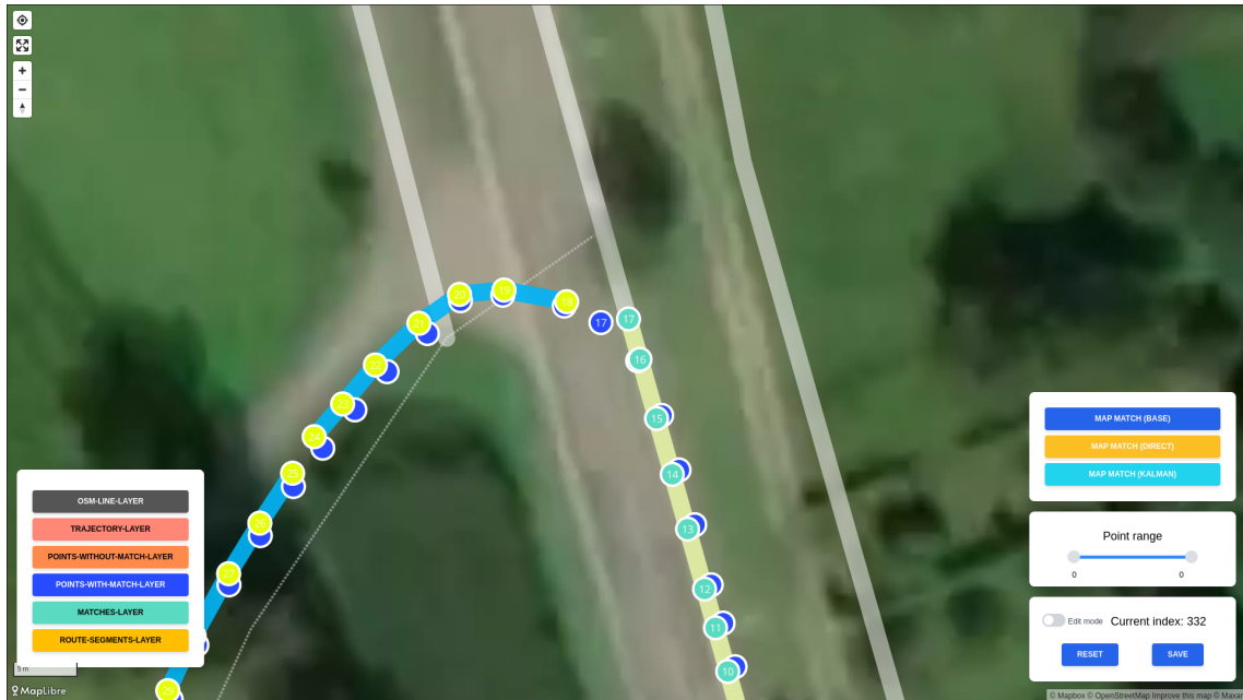
Figure 7.1: Ground truth view for visual and interactive manual map matching. Blue points represent the measured locations, green points are on-road matches and yellow points are off-road matches. Overlaid on top of the satellite base map are the known OSM street in light gray and street segments with randomized unique colors. The bottom left shows controls to hide and show map layers.
