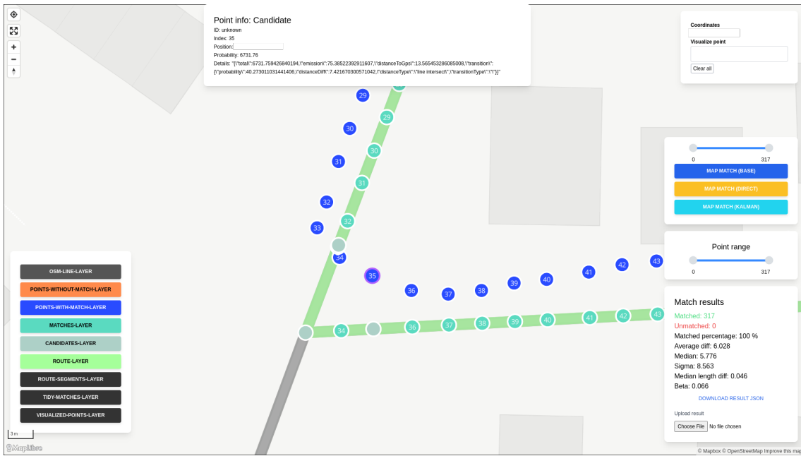
Figure A.9: Visualization view for detailed visual analysis of MM results. Blue points represent the measured locations, green points are on-road matches and gray points are all candidate matches for the currently selected point (purple outline). Detailed information is shown for the MM result in the bottom right as well as for the selected marker in the top. The bottom left shows controls to hide and show map layers.
