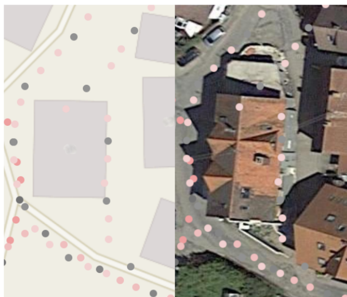
Figure 1.2: An example of an inspected street not being in OpenStreetMap (OSM). The left side shows the OSM base map, contrasted with Google Earth satellite imagery on the right. Overlaid are the measured vehicle location points in red and gray.
