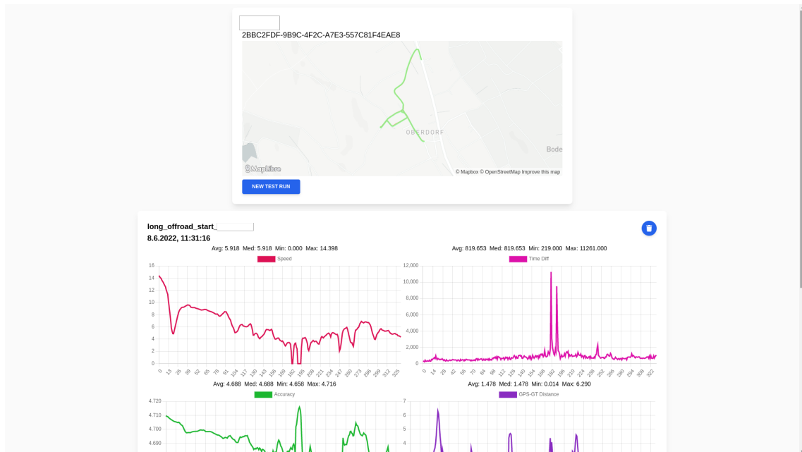
Figure A.10: Inspection test run view for displaying a given inspection with ground truth data, visualizing key metrics as well as triggering MM prototype runs.
